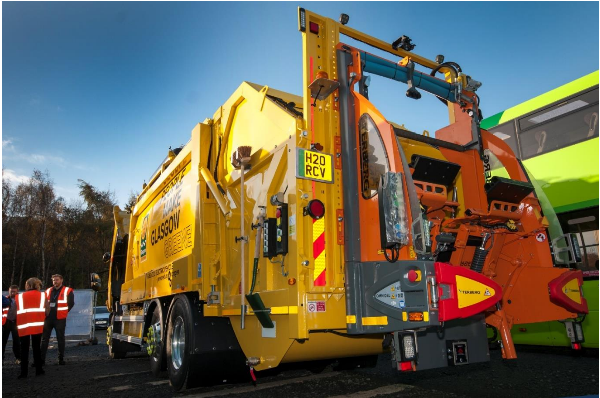
The hydrogen-powered refuse collection vehicle demonstrator developed by Ballard Motive Solutions
