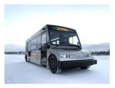
Letenda has chosen to equip its electric buses with the ZEN PLUS battery system, an advanced energy storage solution developed by Forsee Power. The system as applied to the Electrip consists of four ZEN 82 PLUS packs, providing a usable energy capacity of 308 kWh that allows up to 300 km (186 miles) of range. Forsee Power's lightweight batteries combine with the designed-for-electric characteristics of the Electrip for an incredibly efficient vehicle.
